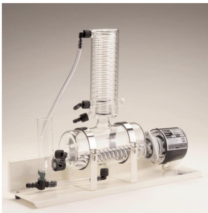
Figure 3-1 Water Still range fitted with metal or silica heater
