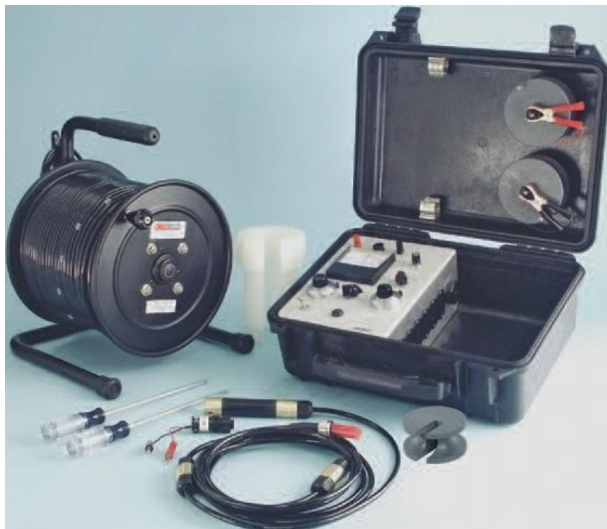
Figure 9-2 Borehole Resistivity System
